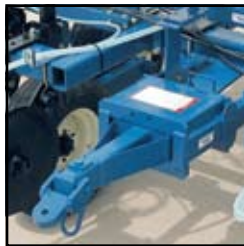
Auto-Lok nurse tank hitch has the largest hitching envelope in the industry, and it retracts for hitching and pulls out to latch.
