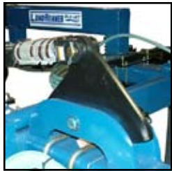
Hydraulic wing cylinder rocker plates provide excellent wing flex.
