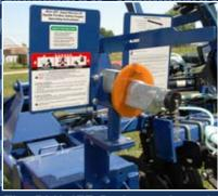
The BLU-JET Bodyguard on the exclusive SuperShooter III helps protect the operator from ammonia spray back during coupling. It features a multi-directional swivel and highly visible operational information
