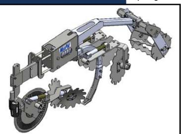
ten inches of trip height resets automatically due to the unique leverages built into the mechanism. And best yet, daily service is not required as greaseless bearing pivot points provide unmatched durability.
